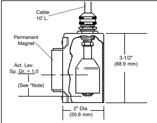
**\*Note:** Switch actuation point is approximately half the distance from end of stem from end of mounting, or at the halfway point of float travel (in liquid with sp. gr. of 1).
