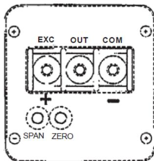
For voltage output, use COM, OUT and EXC terminals.
