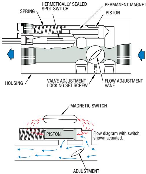
An externally rotatable vane is positioned in the main flow path within the unit. The magnet carrier piston is located in a bypass flow chamber. Pressure differential, caused by flow around the adjusting vane, displaces the spring-biased piston which actuates a hermetically sealed SPDT reed switch within the unit.
