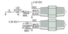
Note: Inductive loads must be diode suppressed.
