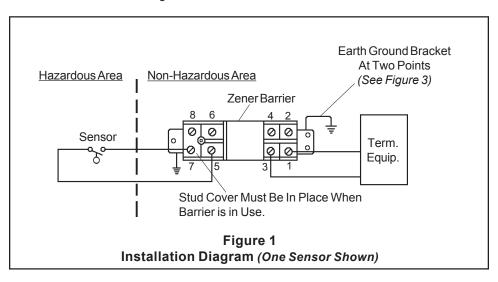
3. The mounting bracket on the barrier must be connected to an earth ground from both mounting points and two lines for redundancy. The grounding should be adequate for conduction of line-generated fault currents. The impedance of either line to earth should be maintained at less than one ohm.
