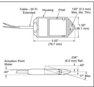
The LS-10's rounded design makes it easy to remove for cleaning and reinstall after an alarm condition is triggered, or for maintenance.
