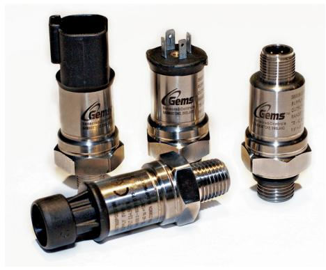
The unwanted areas are removed by sputter etching to create a dielectrically isolated strain gauge in a conventional Wheatstone bridge arrangement, which is mounted on the reverse of a stainless steel diaphragm, resulting in a robust sensor that is suitable for direct contact with almost all liquids, oils and gases.
